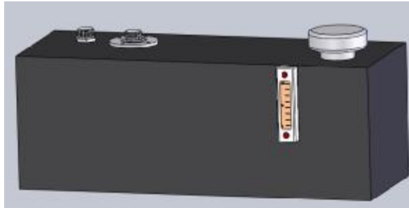
Fig2.3 Hydraulic Oil Tank
